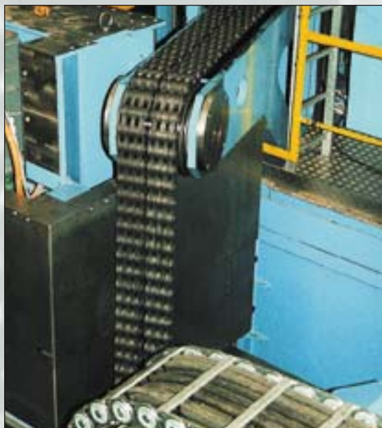
Leaf chains in use in a fork-lift truck (left). Leaf chains (2 x F 76-66) in a machine tool (right).
