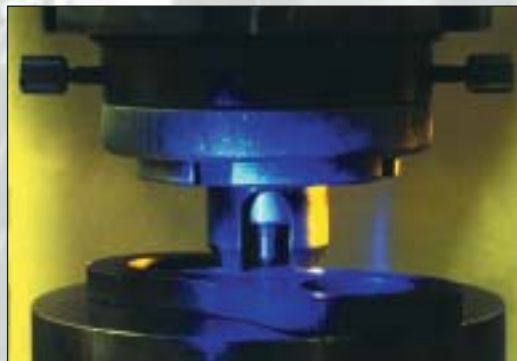
Link plate during Rockwell hardness measurement.
