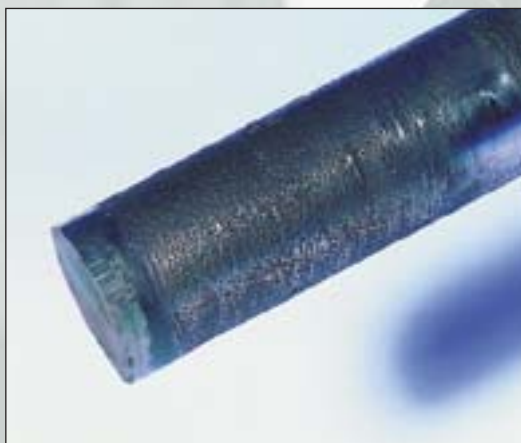
Pitting on pin and plate.
