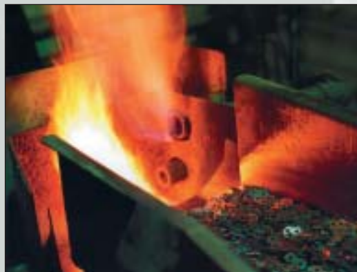
Hardening through heat treatment.
