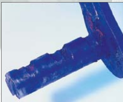
Wear on the chain pin.
